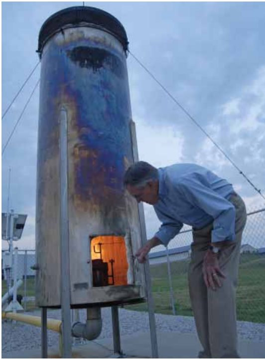
At left: Thomas Butler inspects the flare that burns methane gas created by hog waste. Methane is a formidable greenhouse gas. Burning methane converts it to water and carbon dioxide, which has less heat-trapping power.
