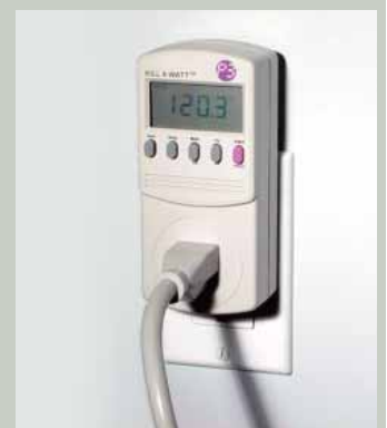
Home power monitors like this Kill-a-Watt model (about $50) are becoming available in home improvement stores and online.
