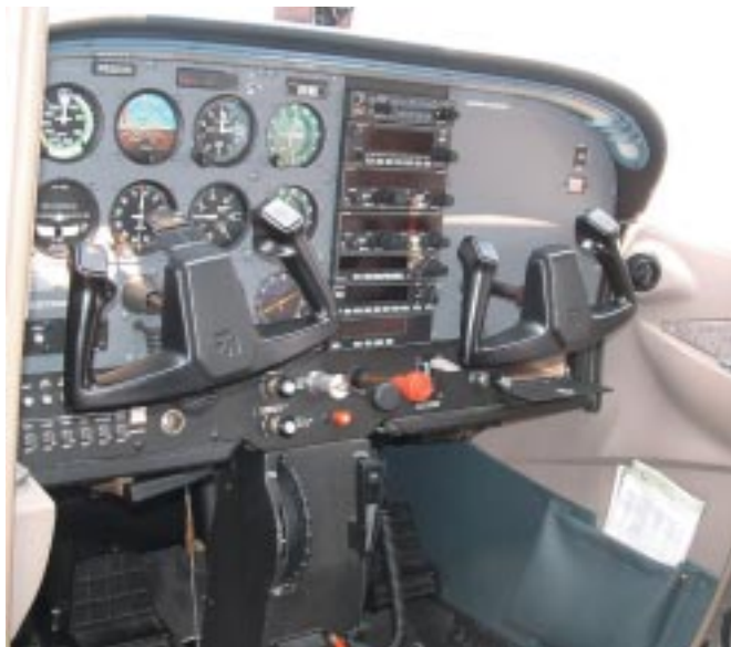
The instrument panel and dual controls of our Cessna 172R. I handled the pilot's yoke on the left (you rotate it like a steering wheel and push or pull it to dip or rise). My instructor had the controls at right, just in case.
