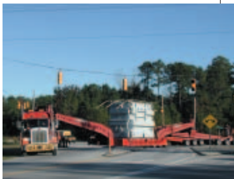
This 74-wheel truck transported one of Brunswick EMC's new transformers to its substation in Grissettown.
