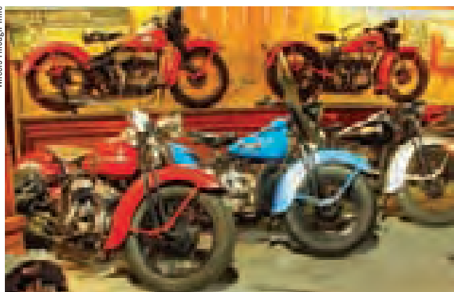
The museum's Harley 45 Exhibit showcases these Harley-Davidson motorcycles with small displacement, lightweight v-twin engines. The machine was appropriately named after its 45-cubic-inch displacement.
